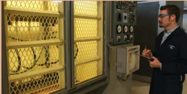
*Gates hose and couplings are pushed to the limit at the world's largest hydraulic impulse test lab, located at the Gates Customer Solutions Center in Denver, Colorado.*
