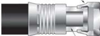
Swivel joint sensitive to over-torquing
