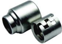
During crimping, only the MegaCrimp coupling’s outside shell takes on the shape of the dies. The “C” insert starts round, stays round – like the hose.
