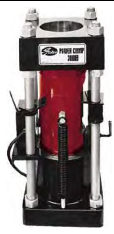
You can use Power Crimp 3000B to couple permanent hose assemblies in hose sizes from 3/16" through 2" (Including 6 spiral). Power Crimp 3000B is rugged enough to absorb the punishment of continued use. The ram can exert a hydraulic force in excess of 125 tons and can crimp all Gates hydraulic hose types, 3/16" through 2".
